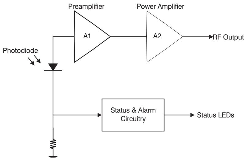
Figure 3.1 Model 2809 Block Diagram
